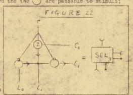
supposed to come from C, goes on to Li, and Lo is isolated from all connections. Hence SCL produces the first state of 13.3 when r is not stimulated, and the second state when r is stimulated. We also note, that in the first case a stimulus passes from Lo to Ly with a delay - (cf. the timing question of SG1, discussed above.)
