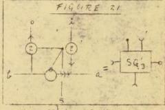
hence b is now connected to a and i to a. Hence  $SG^1$  is on in the sense of 13.2 while s is stimulated, and it is off at all other times. The triple delay on  $\bigcirc$  is necessary for this reason: When  $SG^1$  is on, a
