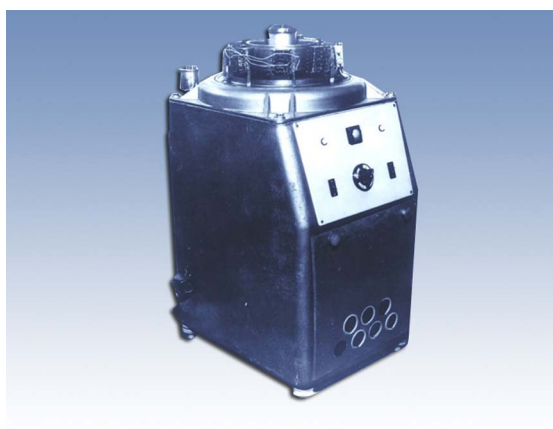
Fig. 6. The drum memory of the M-3. Photo from the CD-ROM supplement of [7].
