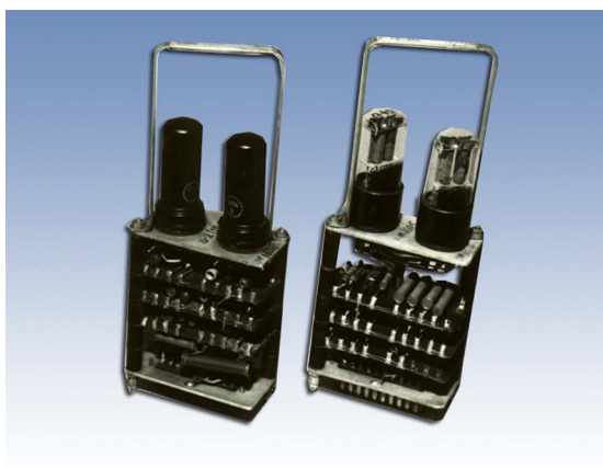
Fig. 2. “The logic units of the M-3 computer. (Left) The new developed drum controller unit, with Hungarian produced long-life tubes. (Right) The old unit; the original Soviet design with Soviet elements” [8, p. 77]. Photo from the CD-ROM supplement of [7].
