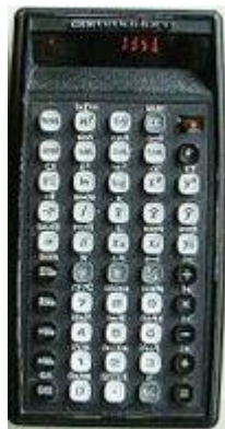
1969: Commodore SR9091SR Texas Instruments chip
