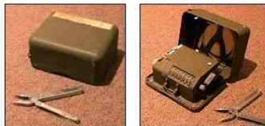
HAGELIN M-209 CIPHER MACHINE (GVG / PD)
